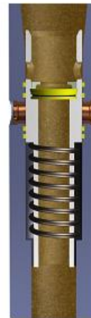
Drilling Mode FLOW to BIT
