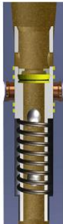
Balls Sheared Thru Seat Tool Reset
