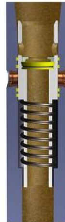
Drilling Mode FLOW to BIT
