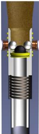
De-Activation Balls Dropped PRESSURE UP
