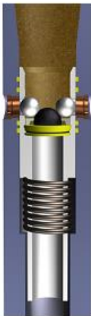
De-Activation Balls Dropped PRESSURE UP
