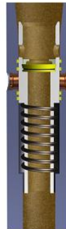
Drilling Mode FLOW to BIT
