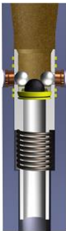
De-Activation Balls Dropped PRESSURE UP
