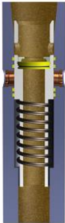
Drilling Mode FLOW to BIT
