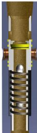
Balls Sheared Thru Seat Tool Reset
