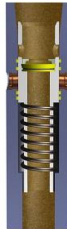
Drilling Mode FLOW to BIT
