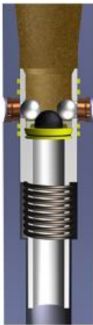
De-Activation Balls Dropped PRESSURE UP
