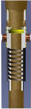
Drilling Mode FLOW to BIT
